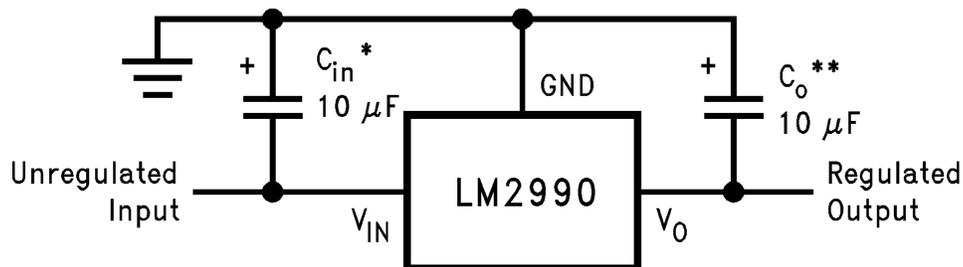
\*Required if the regulator is located further than 6 inches from the power supply filter capacitors. A 1  $\mu\text{F}$  solid tantalum or a 10  $\mu\text{F}$  aluminum electrolytic capacitor is recommended.
