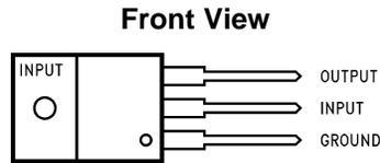
**Figure 1. 3-Lead TO-220 Package**
