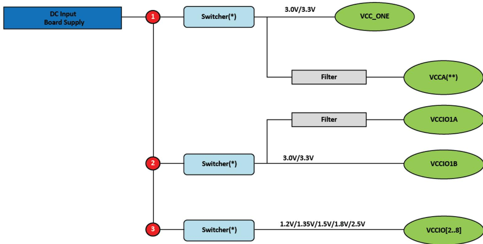
(\*) When using a switcher to supply these voltages, the switcher must be a low noise switcher as defined in *note 9* of the [Notes to Pin Connection Guidelines](#).
