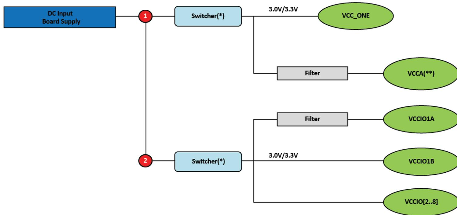
(\*) When using a switcher to supply these voltages, the switcher must be a low noise switcher as defined in *note 9* of the [Notes to Pin Connection Guidelines](#).
