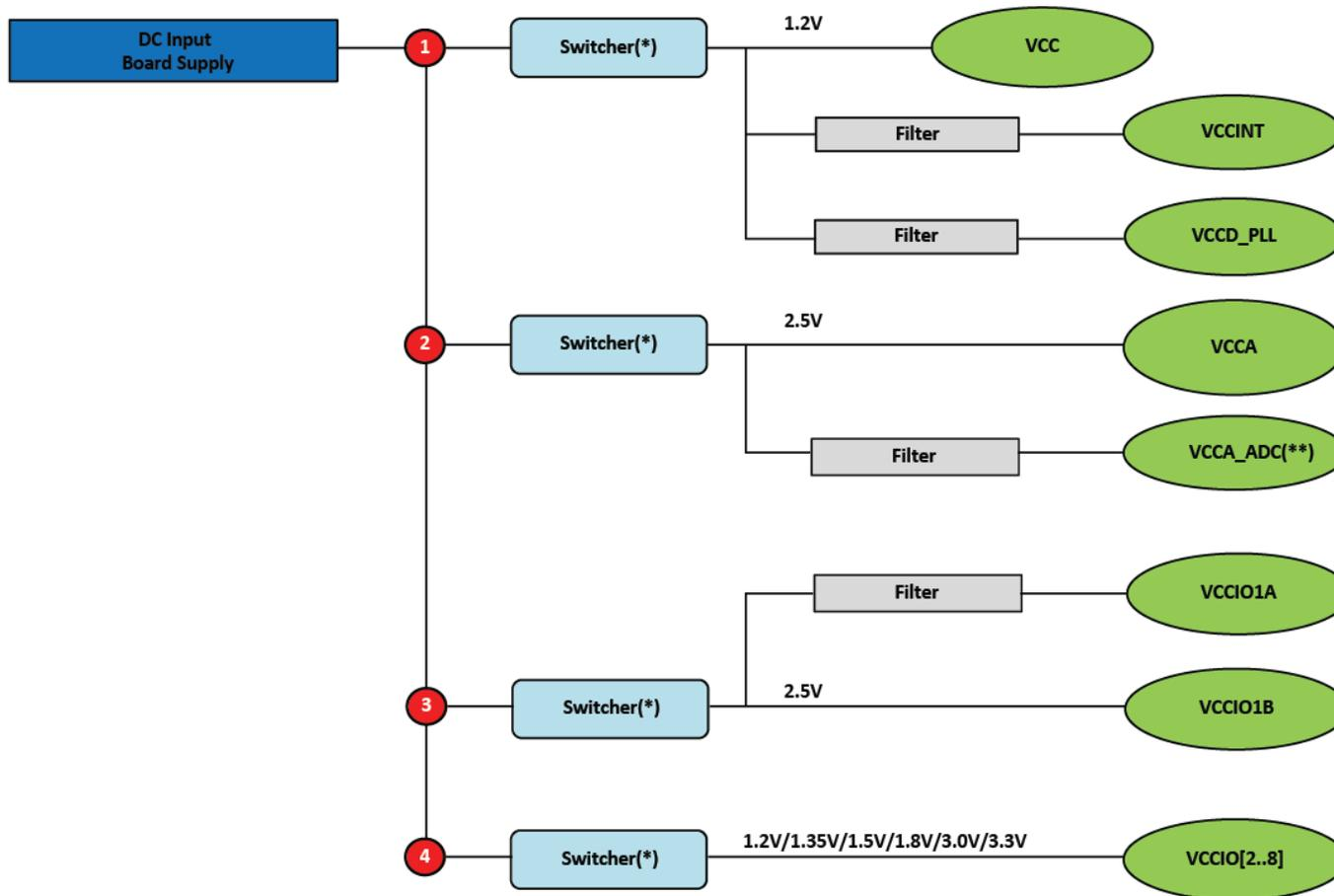
The ADC power supply requires 0.1uF decoupling cap near the package and ferrite bead filter at power supply.
