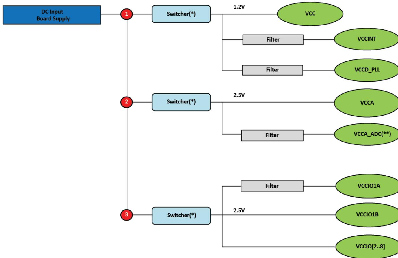
The ADC power supply requires 0.1uF decoupling cap near the package and ferrite bead filter at power supply.
