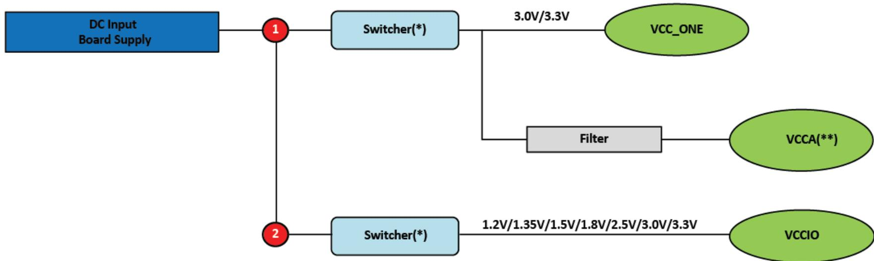
(\*) When using a switcher to supply these voltages, the switcher must be a low noise switcher as defined in *note 9* of the [Notes to Pin Connection Guidelines](#).
