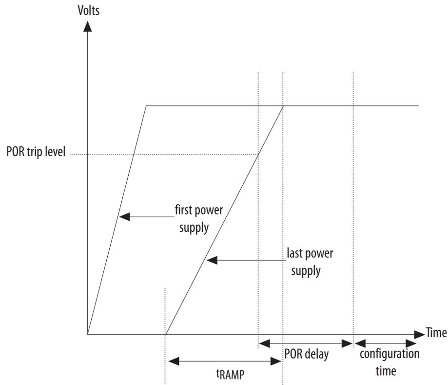
Figure 2-4: Simplified POR Diagram for MAX 10 Devices
