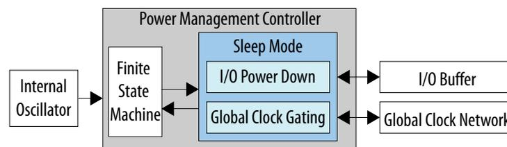
The MAX 10 device contains hardware features that enable I/O power down and global clock (GCLK) gating to manage low-power state during sleep mode. You can power down the I/O buffer dynamically when your application is in idle or sleep mode. One example is the digital single lens reflex DSLR camera
