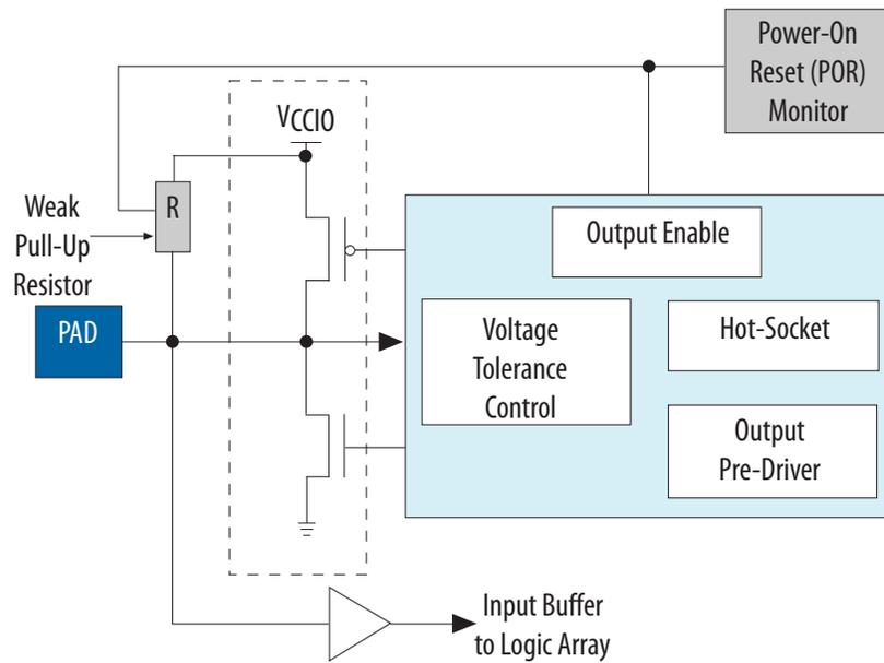
The POR circuit monitors the voltage level of power supplies and keeps the I/O pins tri-stated until the device is in user mode. The weak pull-up resistor in MAX 10 device I/O elements (IOE) keeps the I/O pins from floating. The voltage tolerance control circuit protects the I/O pins from being driven before  $V_{CCIO}$  and  $V_{CC}$  supplies are powered up. This prevents the I/O pins from driving out when the device is not in user mode.
