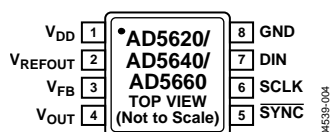
Figure 4. MSOP Pin Configuration
