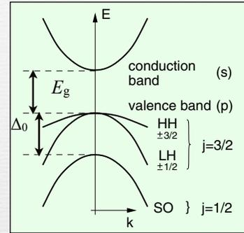
$$H_{S-O} = \lambda \vec{\sigma} \cdot [\vec{k} \times \vec{\nabla} V]$$
