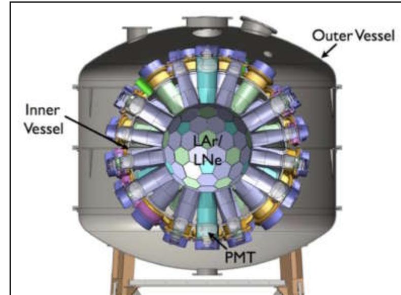
~150 kg fiducial volume (wavelength shifter at  $R=43.5\text{cm}$ , fiducial volume at  $R=30.5\text{ cm}$ )
