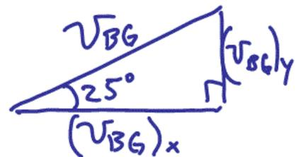
$$(v_{BQ})_x = v_{BG} \cos 25^\circ + 2 = 15.1748 \cos 25^\circ + 2 \\ = 15.75302 \text{ m/s}$$
