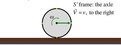
The wheel rotates with angular speed  $\omega$ .
