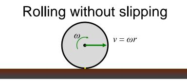
The wheel rotates with angular speed  $\omega$ .
