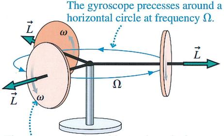
The gyroscope spins with angular velocity  $\omega$ .
