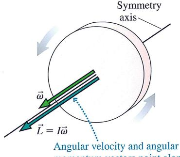
Angular velocity and angular momentum vectors point along the rotation axis in the direction determined by the right-hand rule.
