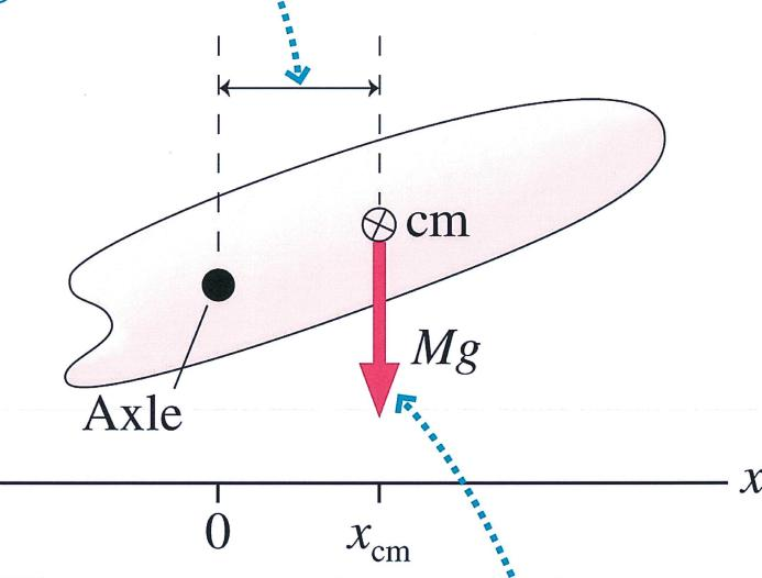
The net torque due to gravity acts at the center of mass.
