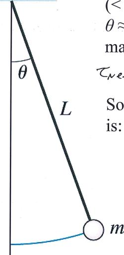
Suppose we restrict a pendulum's oscillations to small angles (< 10°). Then we may use the **small angle approximation** sin  $\theta \approx \theta$ , where  $\theta$  is measured in radians. The net torque on the mass is
