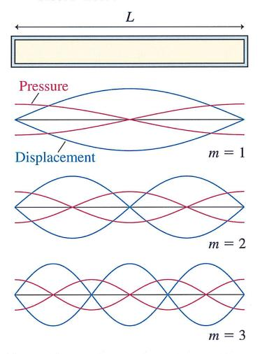
$$\begin{cases} \lambda_m = \frac{2L}{m} & m = 1, 2, 3, 4, \dots \\ f_m = m \frac{v}{2L} = mf_1 & \text{(open-open or closed-closed tube)} \end{cases}$$
