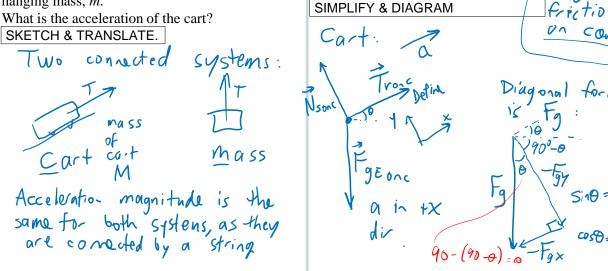
A cart of mass M is on a track which is at an angle of  $\theta$  above the horizontal.
