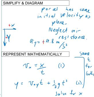
Problem 4.60. An airplane is delivering food to a small island. It flies 100 m above the ground at a speed of 160 m/s. Where should the parcel be released so it lands on the island?
