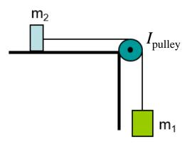
Mass  $m_2 = 2.5$  kg is on a frictionless table. It is attached to a cord that wraps around a massive pulley of radius R = 0.20 m, and rotational inertia I = 0.050 kg m<sup>2</sup>. The same cord is attached to a hanging mass  $m_1 = 0.75$  kg. After the system is released, what is the acceleration of  $m_1$  as it falls?
