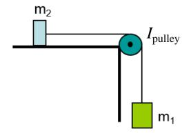
For an accelerating system, the tension must change as it goes over the pulley.
