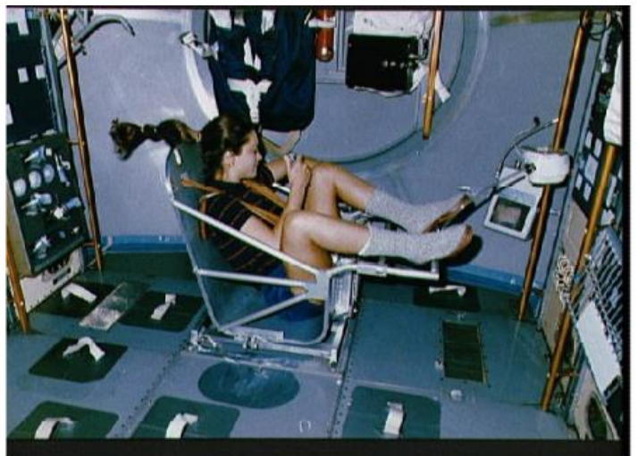
Astronaut Tamara Jernigan (Shuttle Columbia during STS-40, 5-14 June 1991) is weighed into space. This is the first type of "chair pose space." As the chair moves forward and backward, a calculation of the weight counter how astronaut retards the movement of the chair.
