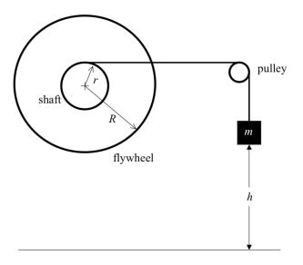
A solid flywheel of radius R and mass M is mounted on a light shaft of radius r so that the axis of rotation is horizontal. A light, inelastic rope is wound around the drive shaft and is connected, via a light, frictionless pulley to a mass m, which is suspended a height h above the floor.
