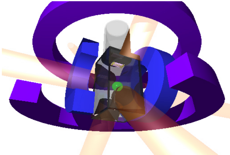
Figure 5: The full experimental setup. This image shows the position of the MOT (central sphere) as well as the MOT and transfer coils, glass vacuum cell, MOT beams and atom chip.
