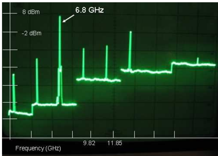
Figure A.8: Spectrum from the output of the 6.8 GHz system (not filtered)
