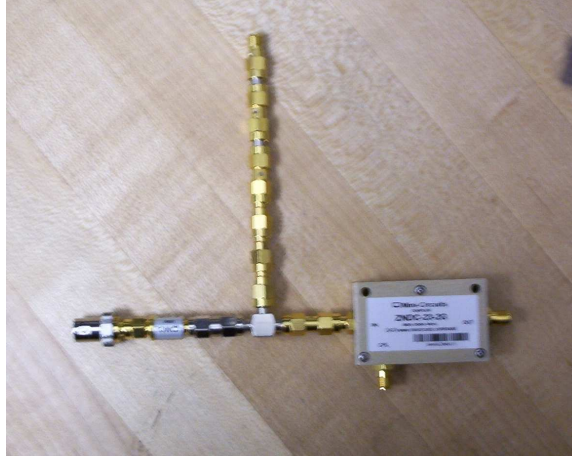
Figure 3.4: Stub used to tune the 1.3 GHz system
