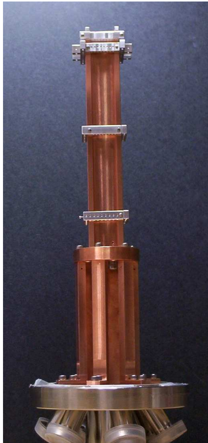
Figure 4.3: The stack (without wires) attached to the vacuum flange
