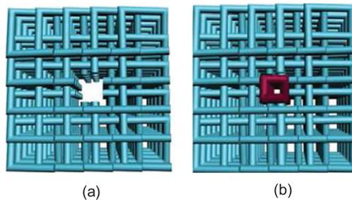
Fig. 6: (Colour on-line) The geometric structures of waveguide in the [001]-diamond: 5 photonic crystal with background spiral parameters of  $[l, c, r, \varepsilon] = [1.6, 1.2, 0.14, 11.9]$ . (a) The waveguide structure formed by drill a cubic block air hole; (b) the waveguide structure formed by inserting a new spiral with parameters of  $[l_w, c_w, r_w, \varepsilon_w] = [0.7, 1.2, 0.16, 15]$  into the air hole in (a).
