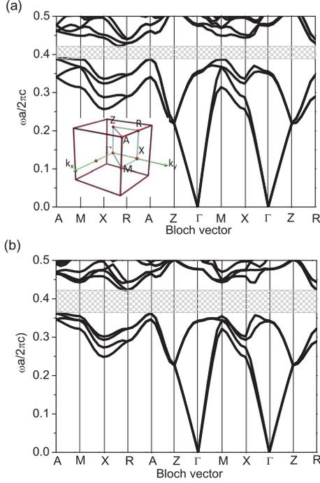
Fig. 2: (Colour on-line) (a) Calculated band structure of the [001]-diamond: 1 photonic crystal with  $[l, c, r, \varepsilon] = [0.72, 1.4, 0.185, 11.9]$ ; (b) calculated band structure of the [001]-diamond: 5 photonic crystal with  $[l, c, r, \varepsilon] = [1.6, 1.2, 0.14, 11.9]$ .
