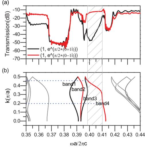
Fig. 7: (Colour on-line) (a) The transmission spectrum of waveguide [001]-diamond: 5 shown in fig. 6 and (b) the corresponding band structure. The black curve is the transmission spectra with incident source  $(E_x, E_y)$  equal to  $(1, e^{\frac{\pi(0+1i)}{2}})$ , and the red curve is with incident source  $(E_x, E_y)$  equal to  $(1, e^{\frac{\pi(0-1i)}{2}})$ .
