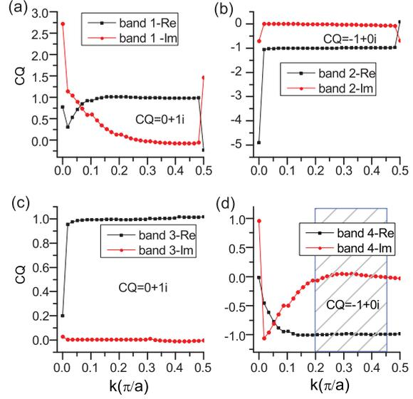
Fig. 8: (Colour on-line) The CQ factors for (a) band 1, (b) band 2, (c) band 3, and (d) band 4. The red dotted line is the real part of CQ, and the black dotted line is the corresponding imaginary part. The shadow region is the WMPG region.
