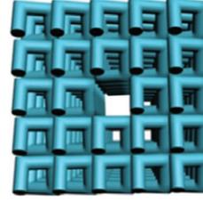
Fig. 3: (Colour on-line) The geometric structure of waveguide in a [001]-diamond: 1 photonic crystal with  $[l, c, r, \varepsilon] = [0.72, 1.4, 0.185, 11.9]$ , which is generated by removing a whole coil of spiral along the  $z$ -axis direction.
