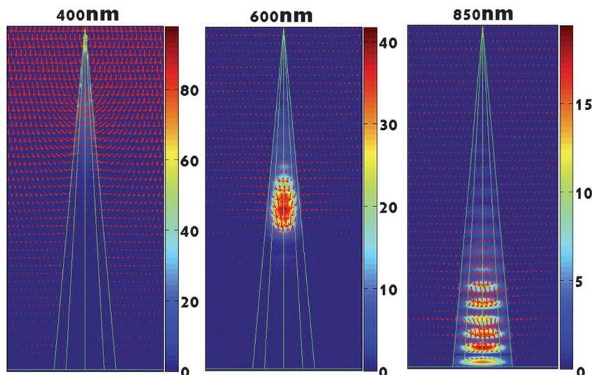
Fig. 10 Orthogonal slice for the Poynting vector and the absorption distribution in gallium arsenide for the 200 nm equivalent bulk thickness conical nanowire photonic crystal (in glass) at three different wavelengths: 400, 600 and 850 nm, respectively. The color bar on the right hand side indicates the intensity enhancement relative to a plane wave with the equivalent input power.
