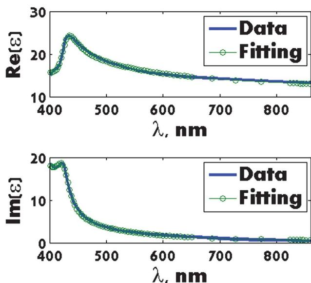
Fig. 11 Fitting of the real and imaginary parts of the frequency dependent dielectric function of bulk crystalline GaAs over the wavelength range from 400 to 860 nm. The solid blue curve represents experimental data<sup>5</sup> and the open circles represent our fit to these data.
