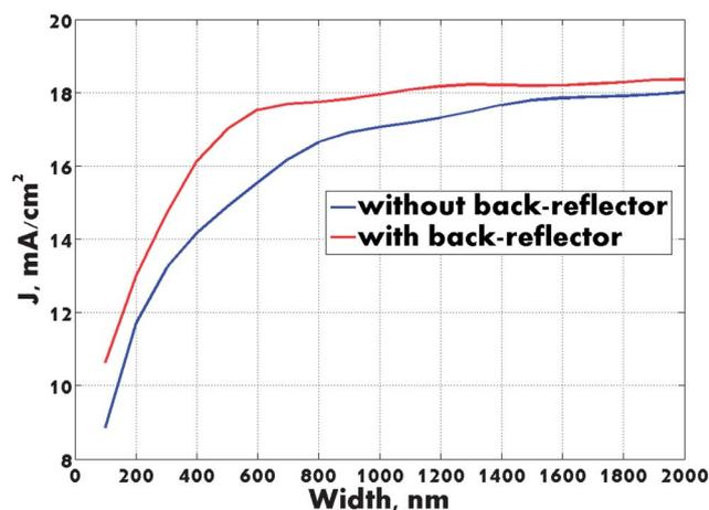
Fig. 1 Maximum achievable photocurrent density (collimated AM 1.5 sunlight at normal incidence) versus the thickness of the GaAs slab with and without a perfect back-reflector in the spectral range [400–860 nm] (red and blue curves, respectively).
