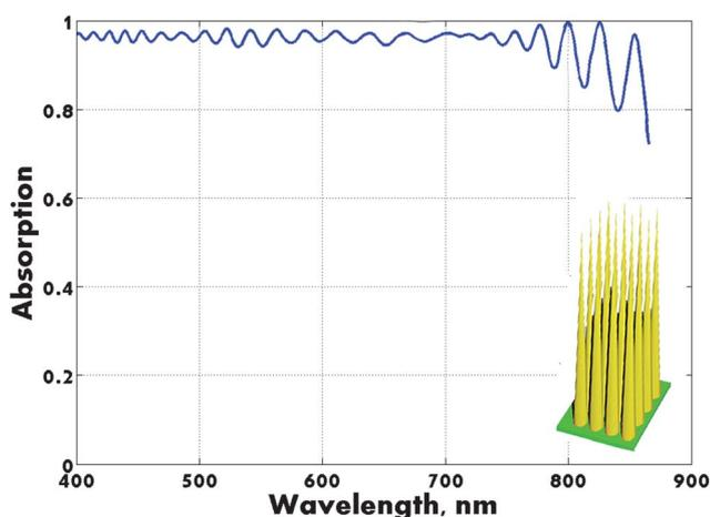
Fig. 8 The absorption spectrum in the range [400–860 nm] obtained for the GaAs photonic crystal made of straight nano-cones, packaged in  $\text{SiO}_2$ , placed on the perfect conductor back-reflector for an equivalent bulk thickness of 200 nm of GaAs. The radius of each cone base is  $r = 100$  nm and the lattice constant is  $a = 500$  nm. The conical nanowire array is depicted in the inset.
