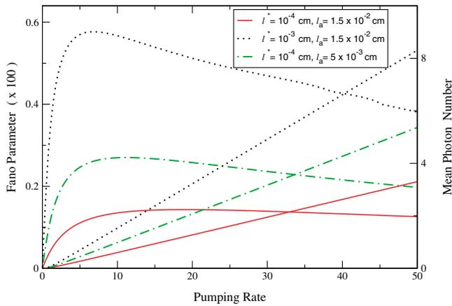
FIG. 2 (color online). Averaged Fano parameter and average photon number for the output radiation, for various scatterer and gain parameters. The other sample parameters are the same as for Fig. 1.
