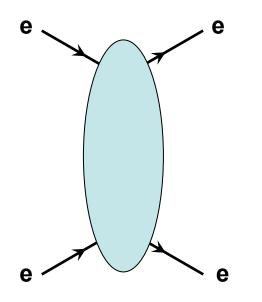
e<sup>-</sup> e<sup>-</sup> → e<sup>-</sup> e<sup>-</sup> (Moller scattering) photon exchange diagram (there is no annihilation diagram)
