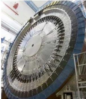
MBTS: minimum-bias trigger scintillator: on inner face of endcap calorimeter
