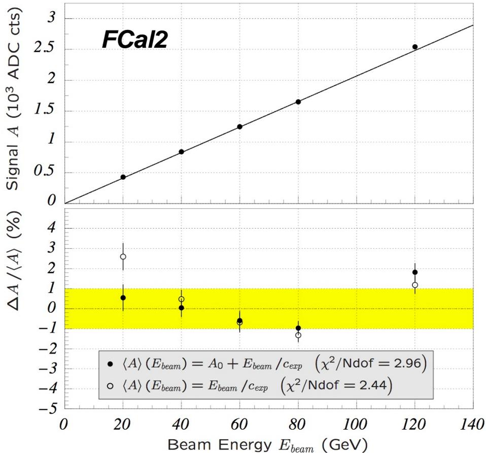
Beam tests in 1998 included separate tests of FCal1 and FCal2 module prototypes with electrons. Allows for the extraction of the ratio of the FCal1 and FCal2 EM Scales
