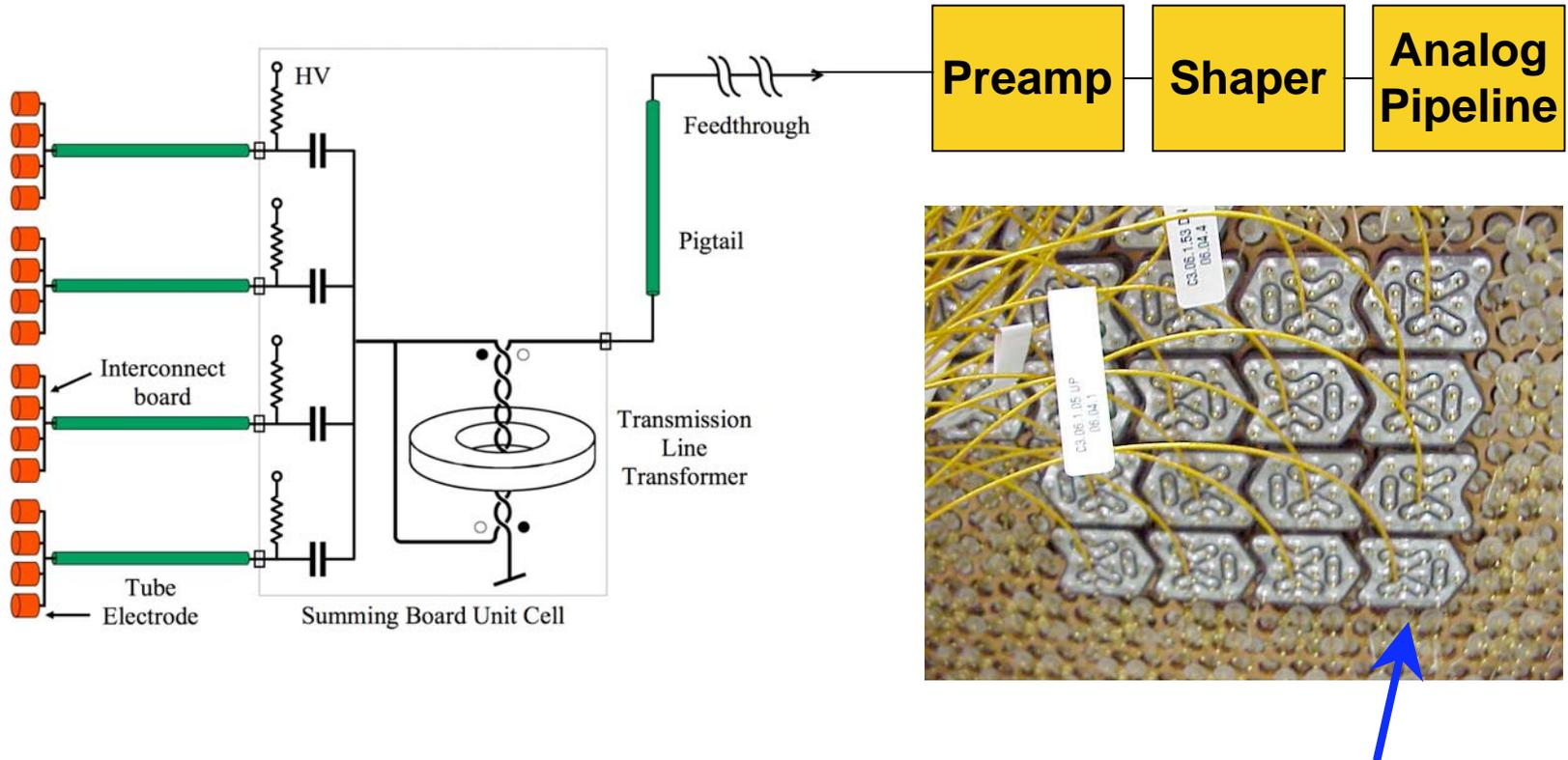
Electrodes are ganged together at module face: 4, 6, and 9 for FCal 1, 2 and 3
