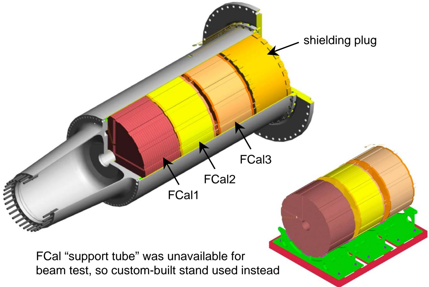
FCal "support tube" was unavailable for beam test, so custom-built stand used instead
