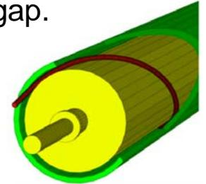
Three modules: 1 EM, 2 Hadronic (ease of construction, depth segmentation)
