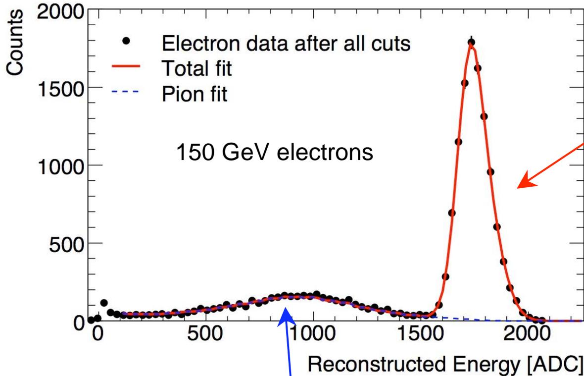
Signal shape non-Gaussian due to impact point dependence of calorimeter response
