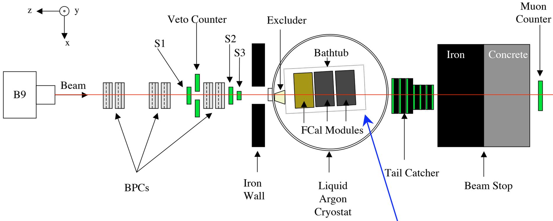
Beamline instrumentation for triggering, tracking: beam cleaning, e/h separation
