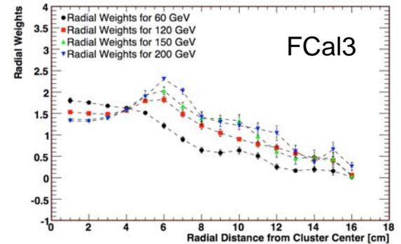
Energy dependence relatively weak for the higher energy samples. Results have been obtained using three sets of weights:
