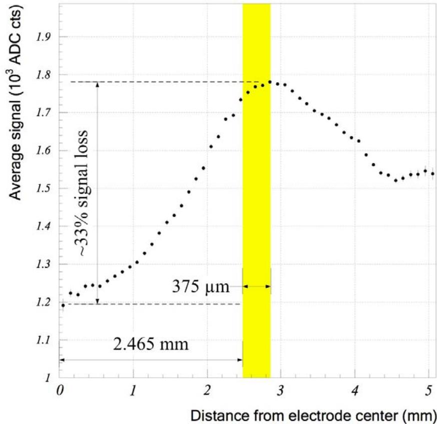
Effect less pronounced in the FCal1 module: trough to peak variation is about 10% rather than the 30% effect seen in the tungsten
