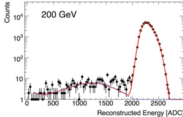
N.B. At 20 GeV fit is DG only. No hadron data recorded at this energy, for modeling of contribution to low energy part of spectrum
