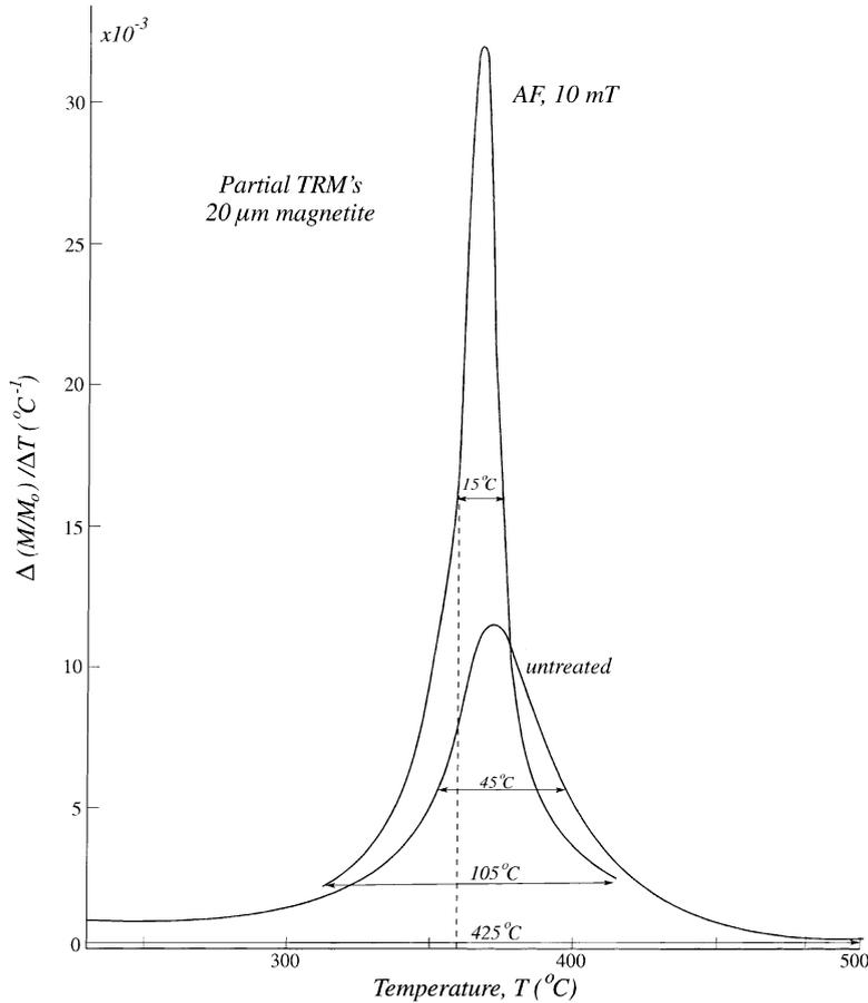
Fig. 7. Unblocking temperature distributions  $f(T_{UB})$  obtained by numerically differentiating the thermal demagnetization curves of Fig. 6. The distribution is sharpened by AF pre-treatment (half-width reduced from 45 to 15°C) and low and high  $T_{UB}$  tails are eliminated (95–5% range reduced from 425 to 105°C). Here magnetization is normalized to post-AF remanence for the AF spectrum, whereas in Fig. 6 normalization was to untreated pTRM.
