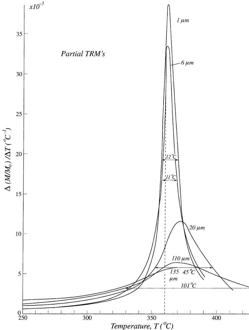
Fig. 3. Unblocking temperature distributions  $f(T_{UB})$  obtained by numerically differentiating the pTRM thermal demagnetization curves of Fig. 2. The half-width of the spectrum for 110 μm MD grains is about an order of magnitude larger than the half-widths for 1 and 6 μm PSD grains.
