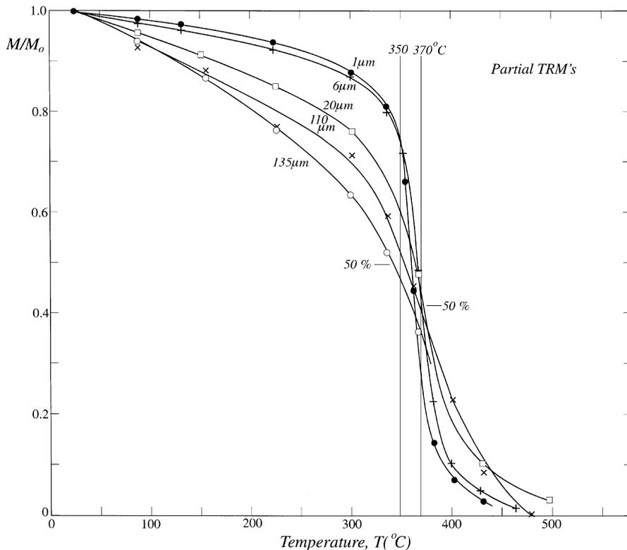
Fig. 2. Stepwise thermal demagnetization of pTRMs produced by a small field applied during cooling from  $370$  to  $350^\circ\text{C}$  in magnetites ranging from small PSD to MD size. About 50–90% of the remanence unblocks at temperatures below or above the pTRM blocking temperature range. These “anomalously” low or high  $T_{UB}$ 's are most important for the largest grains, but are appreciable even for the smallest PSD grains.
