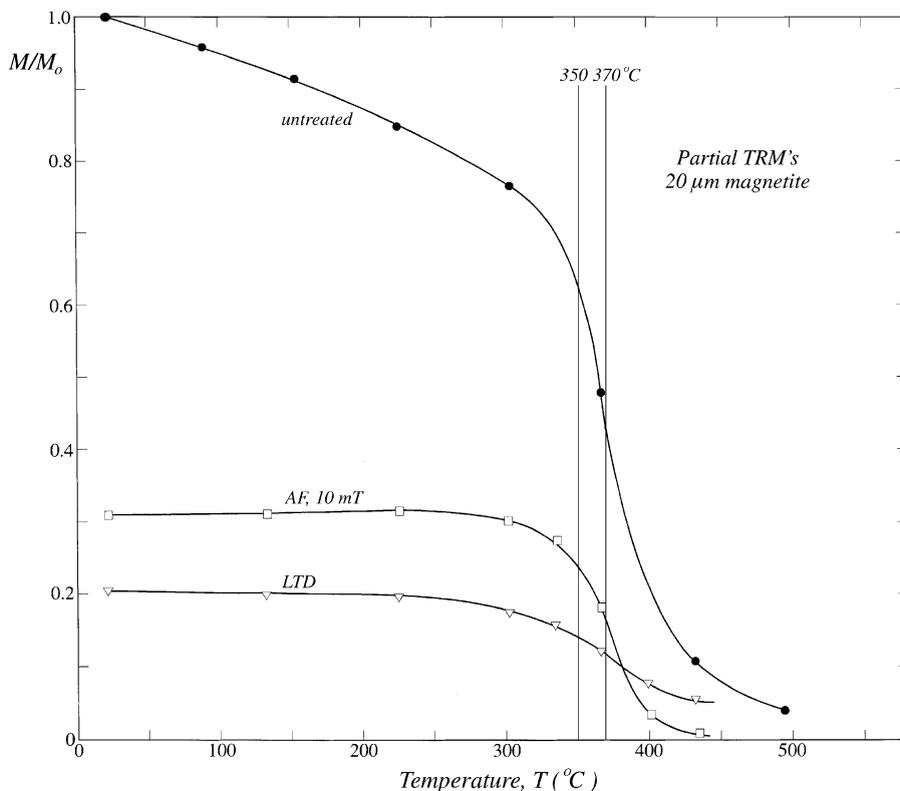
Fig. 6. The effect of AF and LTD pre-treatments on subsequent thermal demagnetization of pTRM for the 20  $\mu\text{m}$  sample. Magnetization is normalized to pTRM intensity before AF or LTD cleaning. AF is the more effective treatment, removing almost all remanence with  $T_{UB}$  outside the 300–400°C range.
