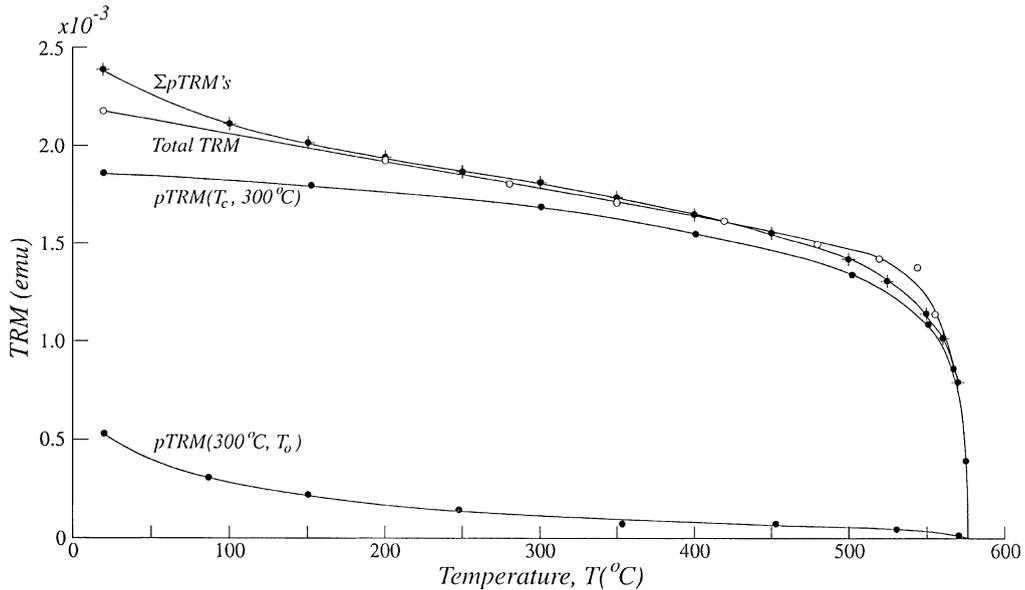
Fig. 9. Additivity of broad-band pTRMs produced over neighboring intervals together spanning the range ( $T_C$ ,  $T_0$ ). At any temperature between about  $100$  and  $500^\circ\text{C}$ , the two thermal demagnetization curves sum to the same value as the total TRM demagnetization curve.
