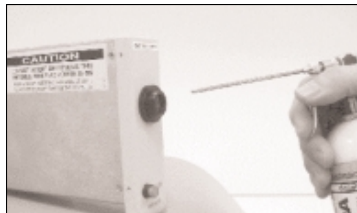
Figure 9b. Cleaning the detector port(s)
