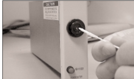
Figure 9a. Cleaning the detector port(s)
