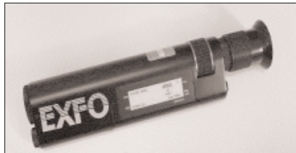
Figure 4. Verify connectors with your FOMS-400X-UNIV
