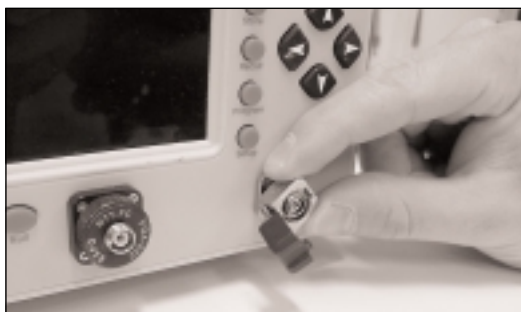
Figure 10. Removing the EUI
