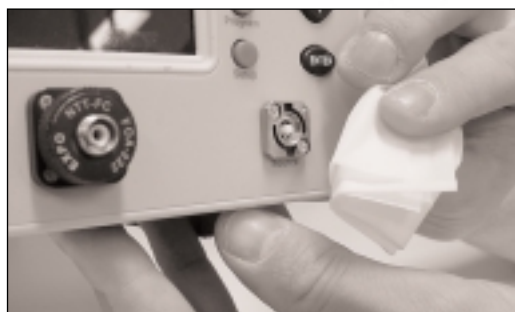
Figure 13. Cleaning the ferrule in the connector port
