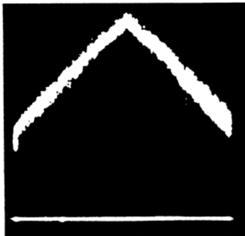
Fig. 2. Autocorrelation of stretched pulse at output of fiber. The pulse is rectangular in shape with a 300 ps pulsewidth.
