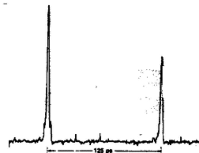
Fig. 4. Streak camera trace of amplified and compressed pulse with a reflection from an etalon. Separation between pulses is 125 ps. Pulsewidth is limited by the streak camera response at 2 ps.
