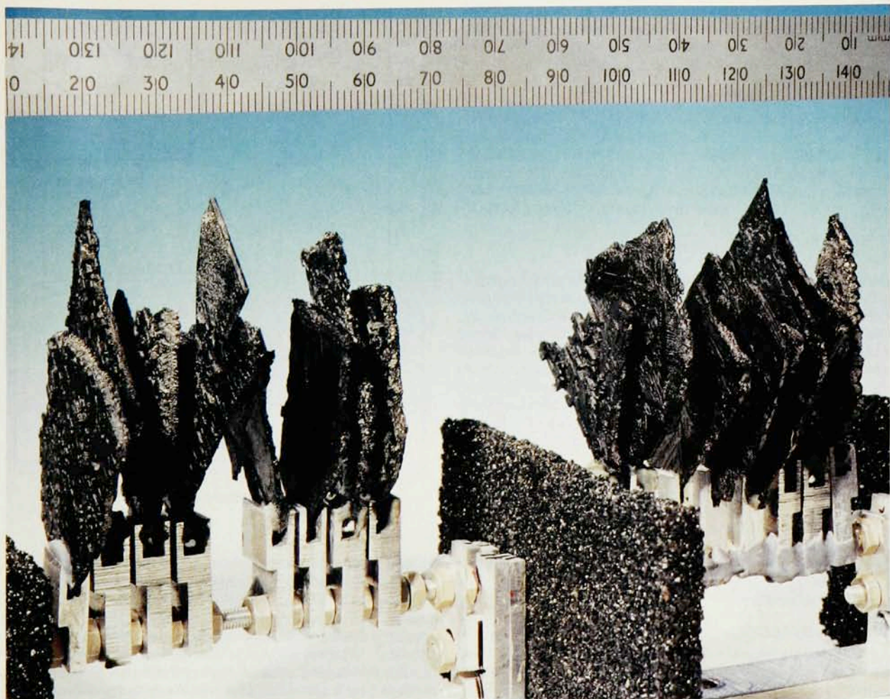
Large \text{La}_2\text{CuO}_4 crystals (the antiferromagnetic parent compound of a family of cuprate superconductors) mounted on a goniometer for inelastic neutron-scattering studies of spin excitations. These plate-like crystals are grown by Sang-Wook Cheong (AT&T Bell Laboratories) and Zachary Fisk (Los Alamos National Laboratory) using \text{CuO}_2 as a solvent (flux technique). The in-plane size reaches up to 8–10 cm. Figure 1
