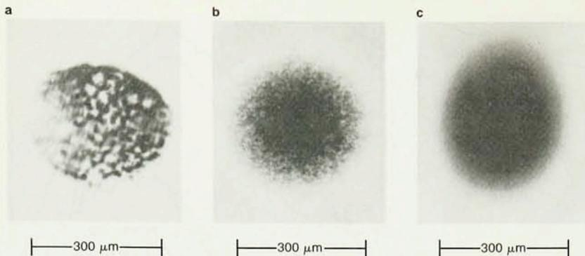
**Beam smoothing.** The images show the time-integrated irradiance profile in the target plane of a nominal 351-nm beam. **a:** The profile from the unadorned Omega laser. **b:** The profile from the random phase plate. **c:** The profile employing smoothing by spectral dispersion. **Figure 6**
