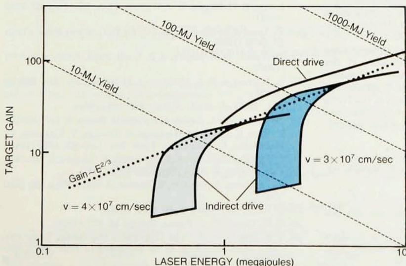
**Predicted target gain** as a function of laser energy for direct- and indirect-drive inertial fusion. The indirect-drive curves are for a fixed coupling efficiency and are parametrized by the capsule implosion velocity. Bands indicate how performance depends on implosion uniformity. Similar hydrodynamic stability criteria are applied to all three curves. **Figure 7**
