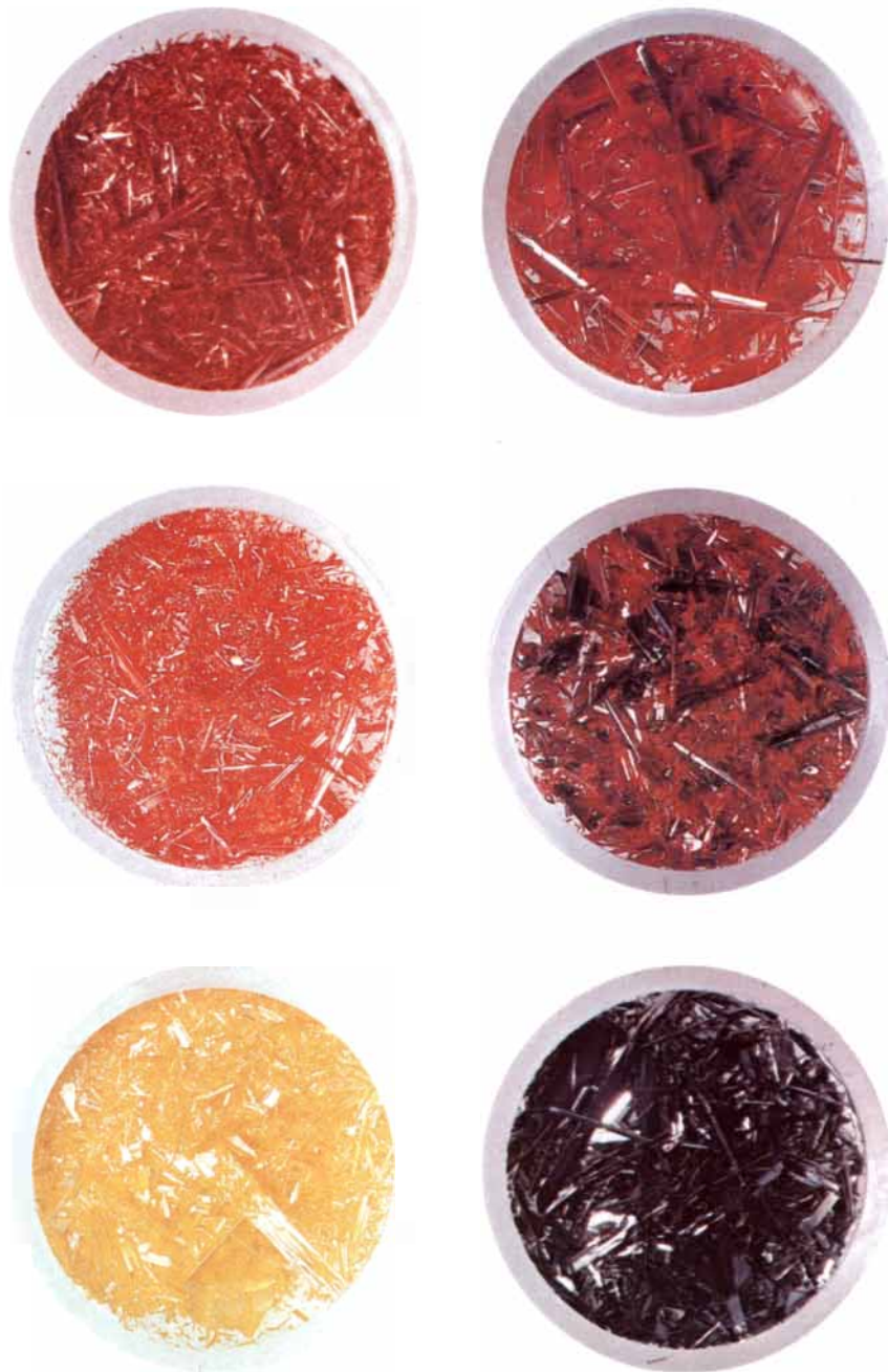
BAND-GAP COLORS are observed in six semiconducting compounds. Pure cadmium sulfide ( bottom left ) has a band-gap energy of 2.6 electron volts, with the result that only violet light can be absorbed; the material has the color complementary to violet, namely yellow. In pure cadmium selenide ( bottom right ) the band-gap energy is 1.6 electron volts, so that all visible wavelengths are absorbed and the crystals are black. The other four materials are mixtures of various proportions of the two compounds; they show a gradient in absorption, with colors from orange through red. The compounds are employed as pigments under the name cadmium red.
