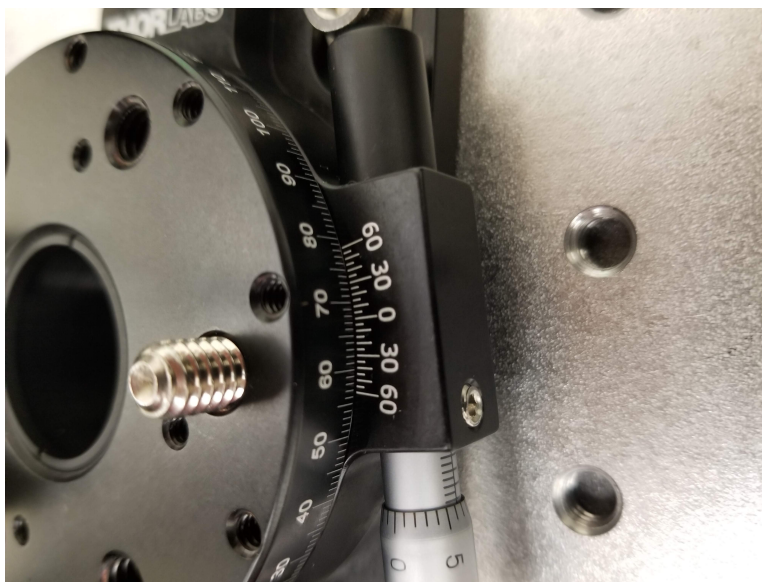
Figure 2: A close-up of the micrometre for the rotation mount. The reading is 67^{\circ}35' .
