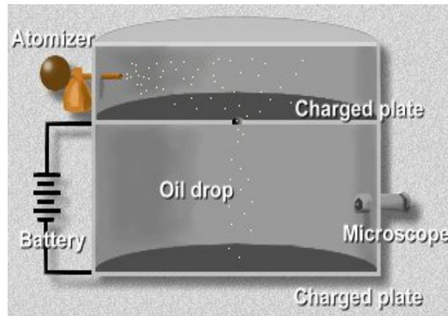
FIG.1: Sketch of a device to produce and observe motion of charged droplets.
