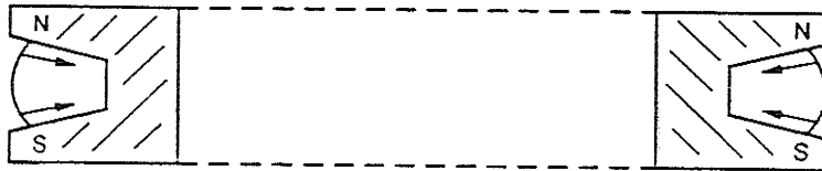
Figure 3.3. Cross section of weak focusing circular accelerator.
