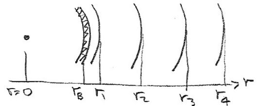
The wires are actually arranged in four layers where they could make very precise ( $\sigma = 150\mu\text{m}$ ) measurements of the  $\phi$  coordinate. The layers themselves were positioned at  $r = 10.0, 11.0, 12.0$  and  $13.0$  cm. For the purposes of this problem you can assume the radially positions of the measurements are at exactly these radii (ie. radial distortions didn't limit this chambers ability to measure the trajectories of tracks emerging from the collisions at  $r = 0$ ).
