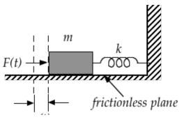
firing of bullets is represented by a general periodic external force (in Newtons) of the form  $F(t) = 25 \sin(60t)$ . The spring opposing the recoil of the bolt provides a linear restoring force, with a spring constant  $k = 2000 \text{ N m}^{-1}$ . Initial conditions are x(0) = 0 m and  $(dx / dt)|_{t=0} = 0 \text{ m s}^{-1}$ .
