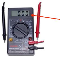
For reading error, generally assume  $\pm$  half of the last digit (meaning  $\pm 0.005$  in this case), *e.g.*
