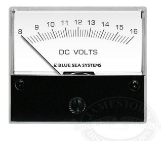
For analog equipment, you are in much the same boat as with a meter-stick. You have to assign a reading uncertainty based on your judgment of how well you can read the device.
