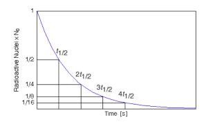
We measure the time of each decay, and then make a histogram of the number of decays in each time bin. One can fit the resulting distribution to the above exponential form to get an estimate of the lifetime  $\tau$  (or do a linear fit to a log plot....).
