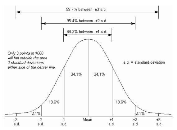
For Gaussian distributed uncertainties, expect that a given measurement should fall within  $\pm 1\sigma$  of the "true" value 68.3% of the time, within  $\pm 2\sigma$  95% of the time, within  $\pm 3\sigma$  99.7% of the time.....usually quote  $1\sigma$  errors.
