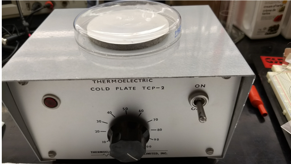
Figure 7. Thermoelectric cold plate and the petri dish used as a cover. The cover is used to keep the air inside the petri dish more or less stable.
