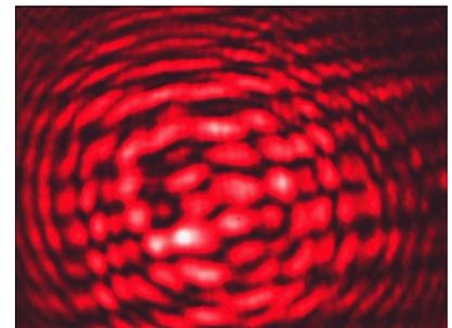
Now adding pinhole interferometer, to measure wavefront curvature
