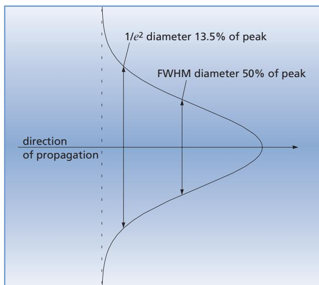
Figure 2.2 Diameter of a Gaussian beam
