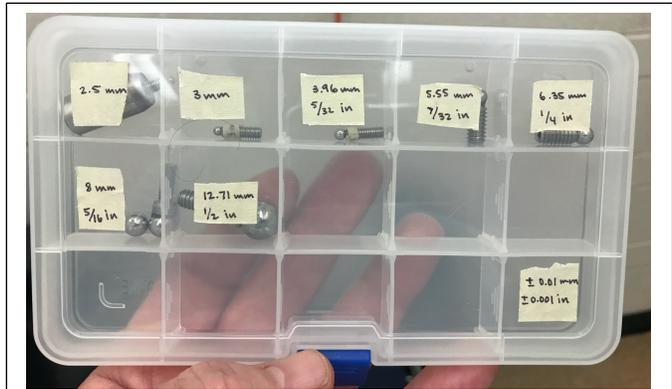
Mounted steel balls: spherical reflectors.
