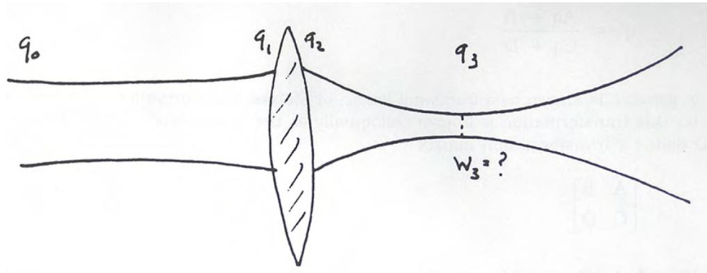
Fig. 2: Focussing a Gaussian laser beam
