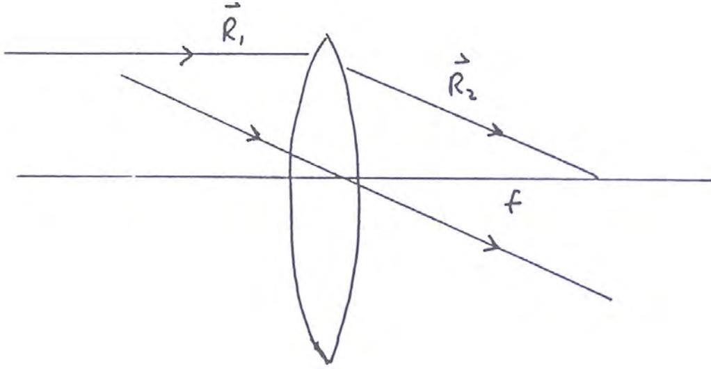
FIGURE 6.1.2. Ray transformation by a simple lens.
