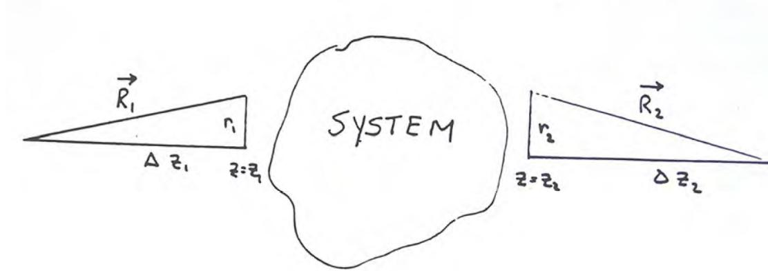
Fig. 3: Rays entering and leaving an optical system.
