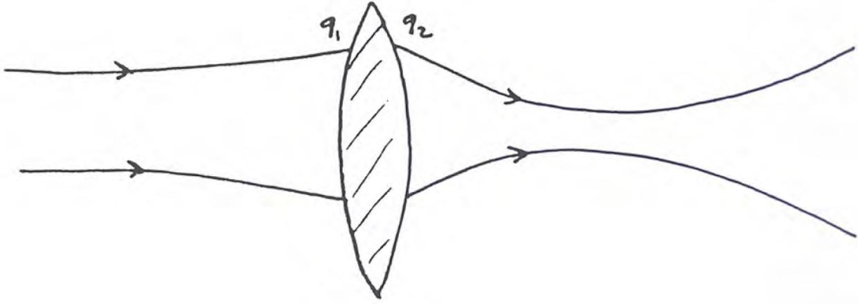
Fig. 3: Transformation of a Gaussian beam by a lens.
