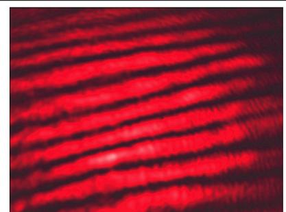
Planar interference fringes between two slightly angled HeNe beams
