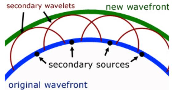
Huygen's construction predicts the new wavefront after propagating a little distance. Fresnel took it further, and literally: the new wave is the mathematical sum, the net interference, of all the little wavelets, *including phase*.
