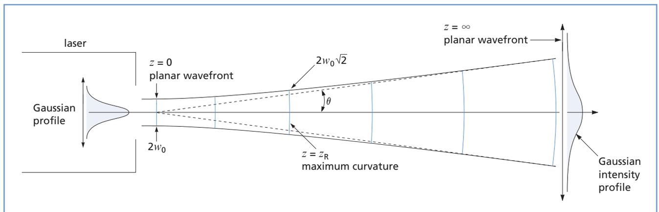
Figure 2.4 Changes in wavefront radius with propagation distance
