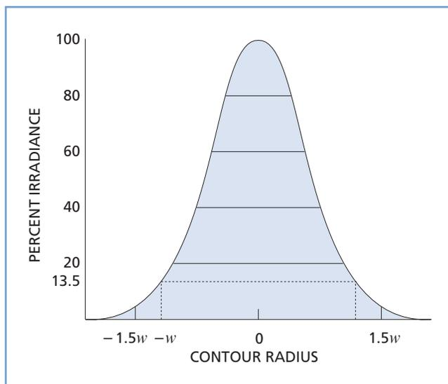
Figure 2.1 Irradiance profile of a Gaussian TEM<sub>00</sub> mode
