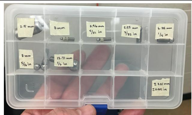
Mounted steel balls: spherical reflectors. Consider also the mounted glass balls, especially also high-quality (better than  $\lambda/10$ ) spherical-surface glass lenses of different focal length (provided).
