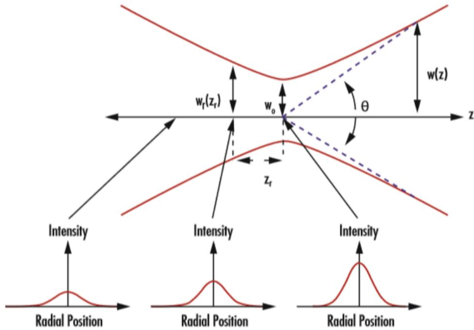
Fig. 5. Schematic of a gaussian beam: This figure makes clear that the hyperboloids which trace the  $1/e$ -max surfaces are not surfaces of constant intensity, but just mark the width of the diminishing profile.
