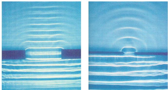
Wave-tank illustrations show how plane waves spread, or diffract, beyond an aperture. Smaller apertures  $\Delta x$  result in a bigger lateral spread  $\Delta k_x$  of wavevectors, which tie to momentum.
