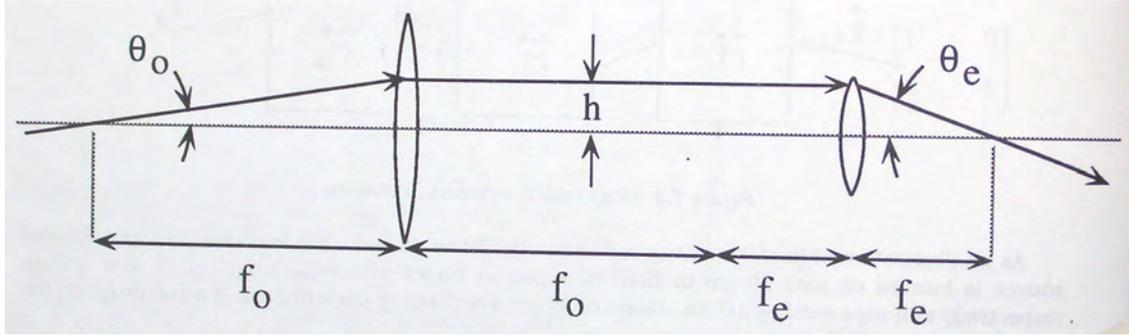
FIGURE 6.3.1. Astronomical telescope
