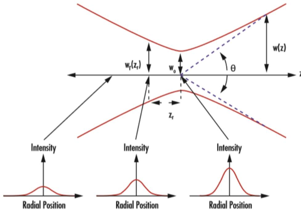
Fig. 2: This figure makes clear that the hyperboloids which trace the 1/e-max surfaces are not surfaces of constant intensity, but just the ‘shoulders’ of the profile.
