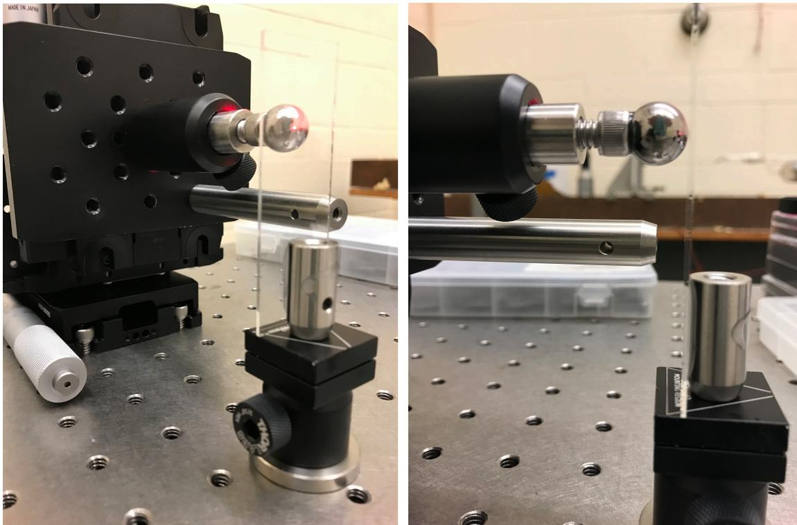
Fig. 4. One method for referencing absolute z-position in space: special mount with microscope slide – the reflected laser beam is very sensitive to the moment the ball touches the glass.
