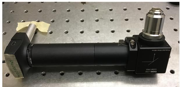
Beam microscope. The USB camera connected can be controlled and analysed using ImageJ software. Calibrate by moving the microscope sideways a distance measured on micrometers, and comparing to movement of the image on the camera.
