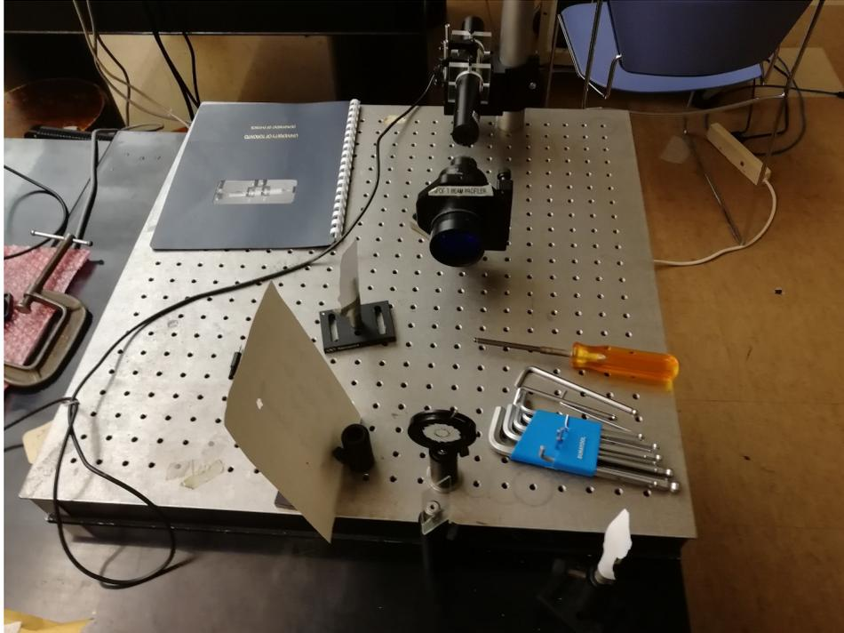
Fig. 3. An image of the HeNe laser into a beam expander and then into an iris. The painted iris allows for users to determine the position of the collimated beam, with the beamsplitter (microscope slide) in front of the iris, also contributing to user's ease in determining the collimated beam size.
