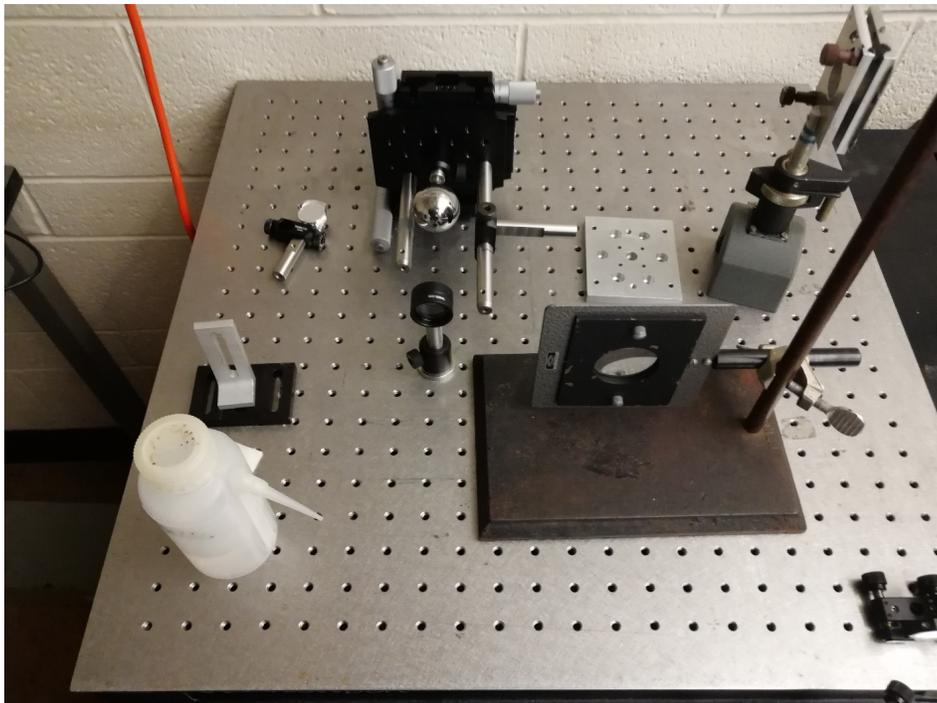
Fig. 2. An image of the steel balls attached to the translation stage setup with various lenses. Three separate translation stages allow for full control in the  $x,y,z$  planes at the micro scale.
