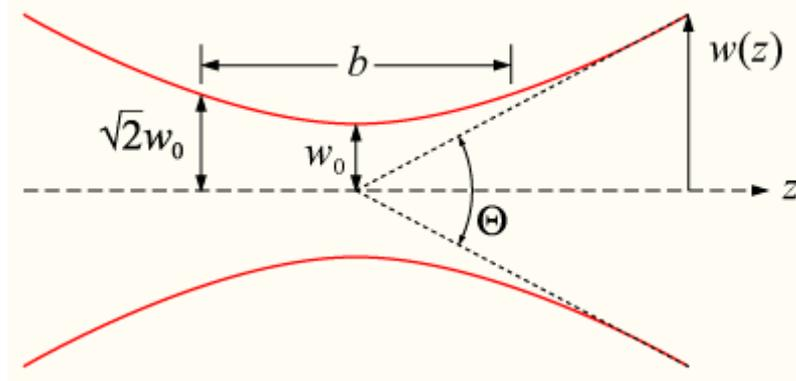
Fig. 1: Surfaces of constant spot size  $w(z)$  follow hyperboloids of revolution, according to Eqn. 17. Note that like a FWHM measurement,  $w(z)$  – the half-width 1/e-max of the  $E$ -field – is measured relative to the peak. But the peak decreases in either direction as one goes away from the beam-waist at  $z=0$ .
