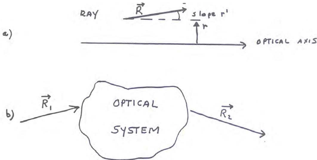
FIGURE 6.1.1. Transformation of a ray by an optical system.
