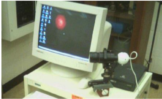
Figure 2: Camera and computer to measure beam profile
