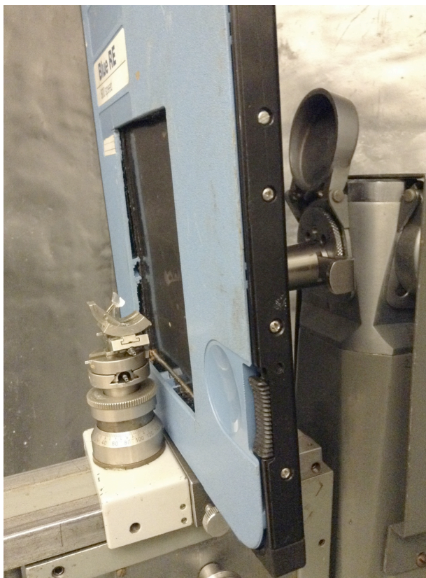
Figure 9: Crystal mounted on goniometer in front of Camera on the X-ray Machine.
