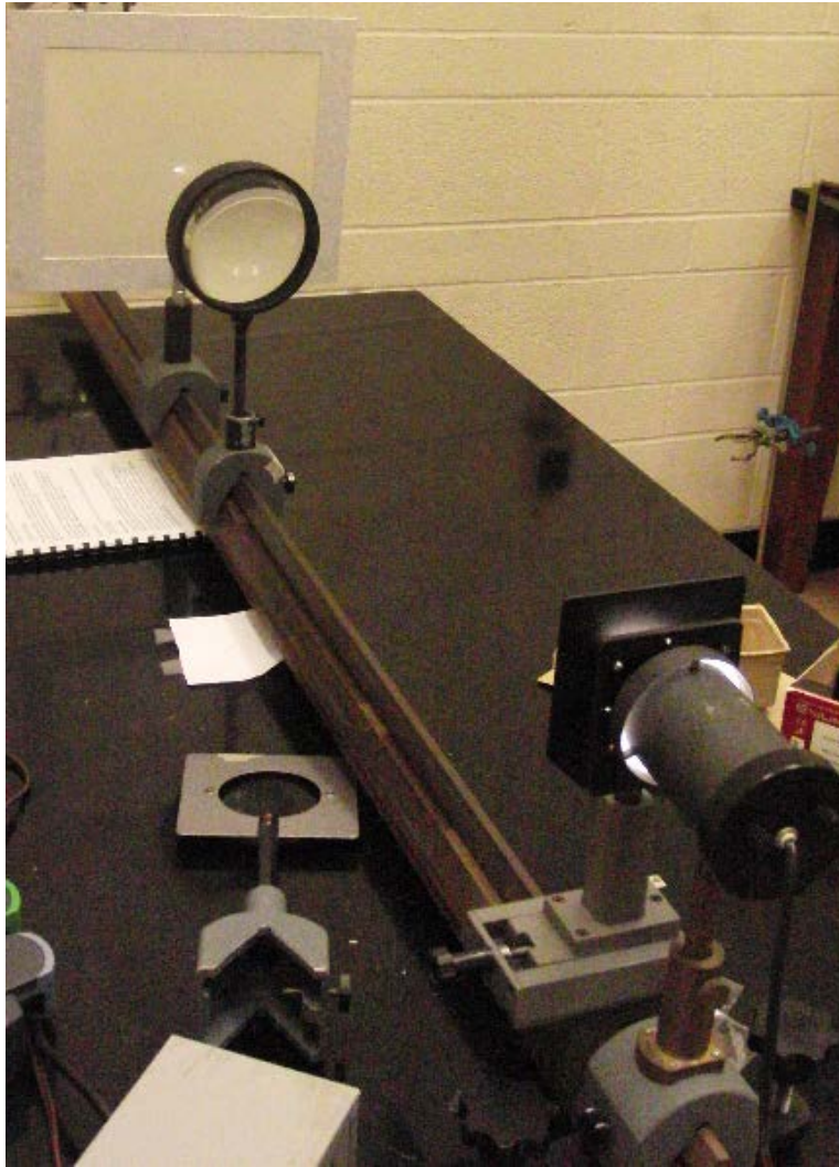
Fig.5. Possible alignment of the setup for coma observations.
