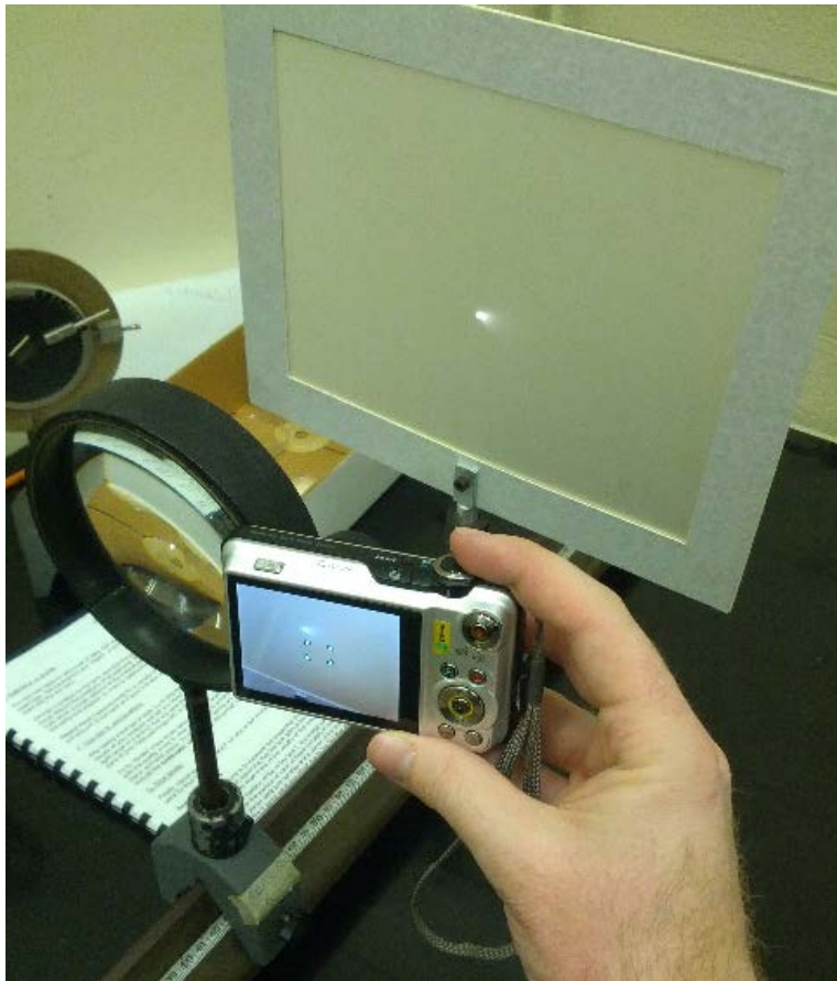
Fig.6. Observation and photographing coma on the screen in experiment LENS.
