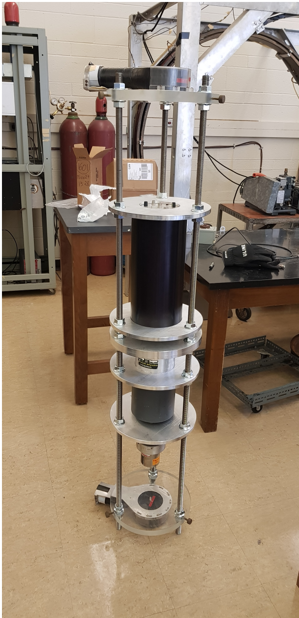
Figure 7: The assembled full muon telescope before mounting on rotating stand. Scintillators from top to bottom are: pancake, plastic, NaI, pancake scintillator
