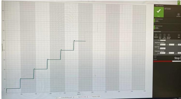
Figure 6: Work sequence for the heating stage. Notice that the delta and slope are causing delay in every cycle to ensure the temperature fluctuation is controlled.
