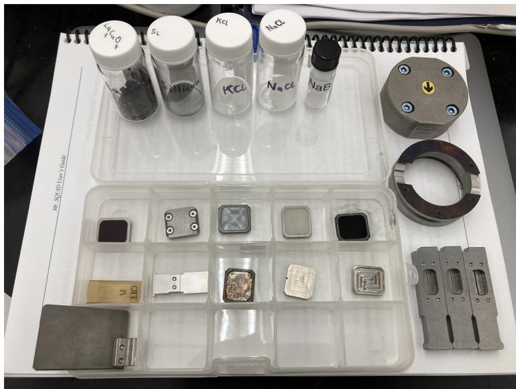
Figure 5: Required materials: Five powder samples in bottles, heating stage sample holders in the box with knife edges. The standard calibration slit block, single sample holder and three divergence slits on the left.
