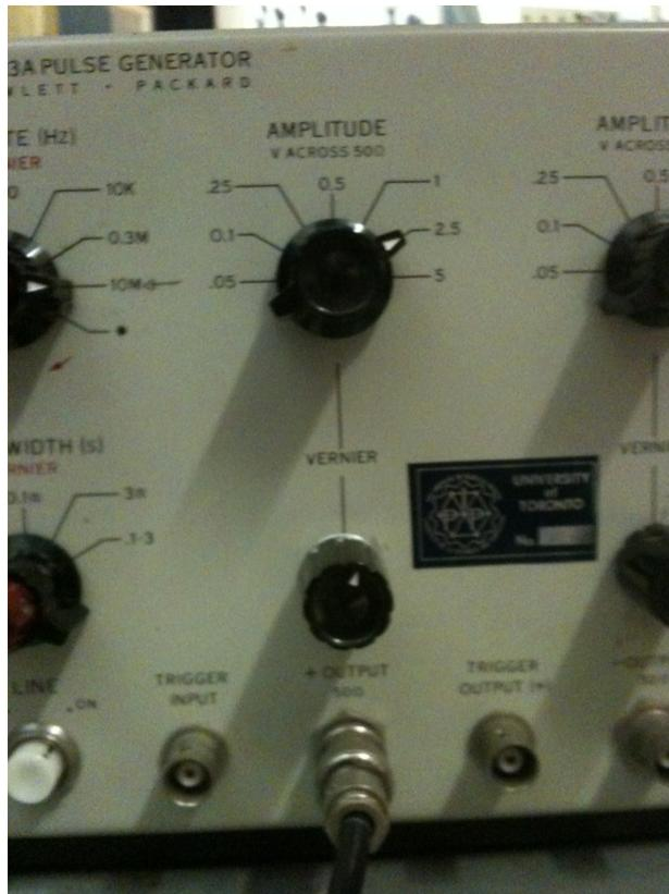
Figure 3 - Knob settings for pulse generator
