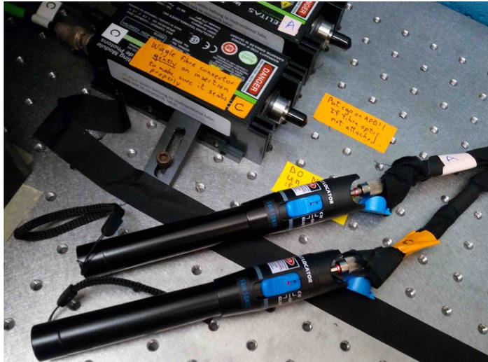
**Figure 5:** Both fibre optics inserted into visible fault detector. Note that the APD inputs are properly capped.
