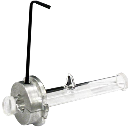
Figure 5 9 mm Adapter Mounting onto Gas Cell
