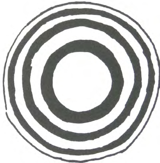
FIGURE 8.4.7. Fresnel zones for a circular aperture with the observation point on axis.
