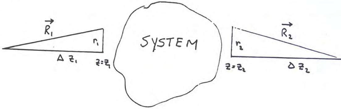
FIGURE 10.6.3. Rays entering and leaving an optical system.
