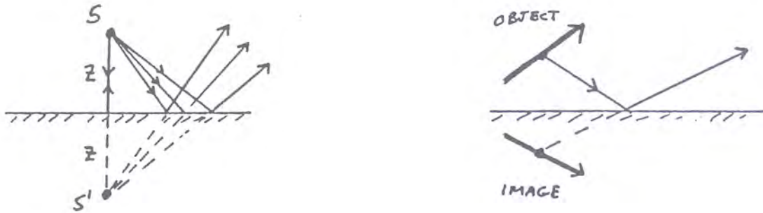
FIGURE 5.2.2. Image formation of a plane mirror.
