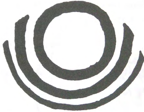
FIGURE 8.4.8. Nature of the Fresnel zones inside a circular diffracting aperture when the center of the zones at P_m is not at the center of the aperture. The contributions from adjacent zones is of opposite sign and nearly cancel.
