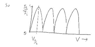
The voltage which provides maximum transmission is the half-wow voltage, which cause the Pockets cell to rotate the incident polarisation through 90°.
