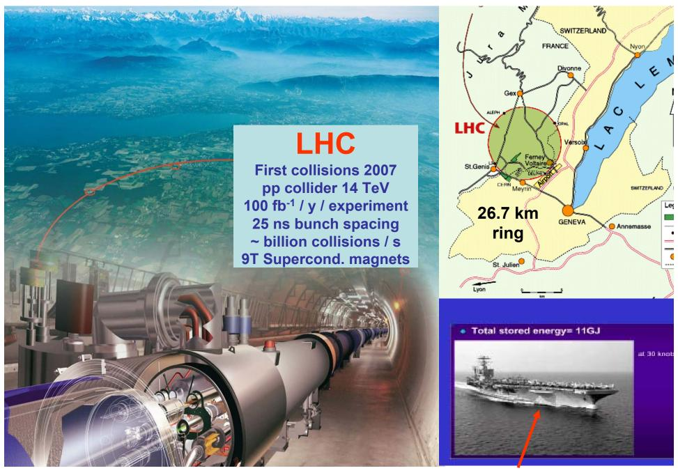
Energy (2 LHC beams) = 11 GJ = 7% of energy stored in an aircraft carrier at 30 knots
