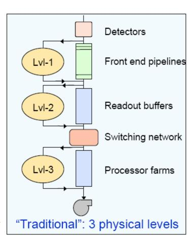
Complicated Example: Trigger / DAQ for the ATLAS Experiment at CERN
