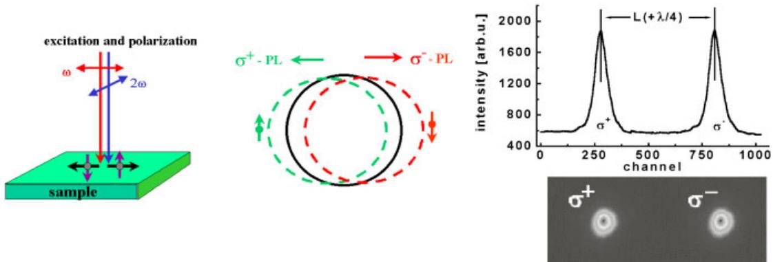
**Fig. 3** (online colour at: [www.interscience.wiley.com](http://www.interscience.wiley.com)) Determination of the PL-spot positions for  $\sigma^+$  and  $\sigma^-$  polarization.
