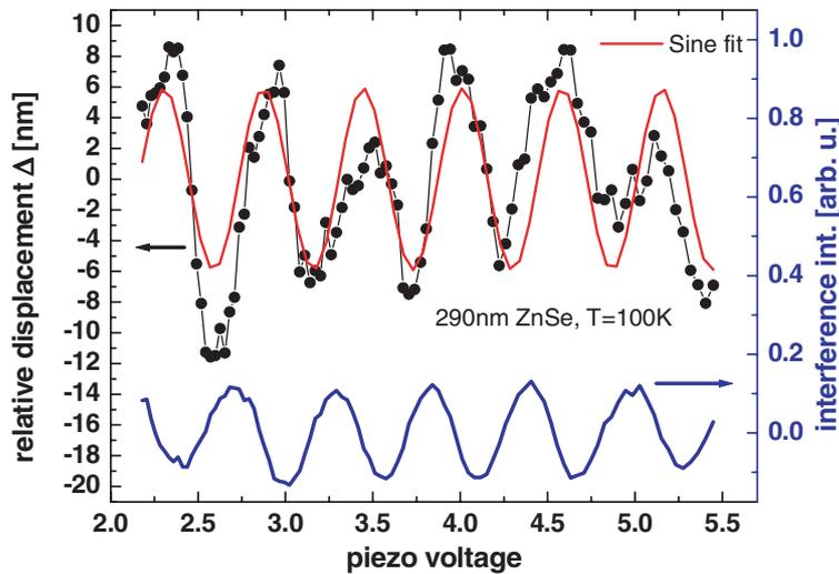
**Fig. 4** (online colour at: [www.interscience.wiley.com](http://www.interscience.wiley.com)) Relative displacement  $\Delta$  of the  $\sigma^+$  and  $\sigma^-$  polarized PL spots (upper part) and the intensity of the interference of the frequency-doubled  $\omega$  with the  $2\omega$  laser beam after the cryostat (lower part) as a function of voltage applied to the piezo crystal in the Michelson interferometer.
