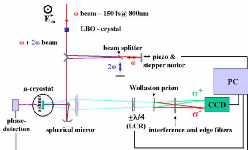
**Fig. 2** (online colour at: [www.interscience.wiley.com](http://www.interscience.wiley.com)) Experimental set-up.
